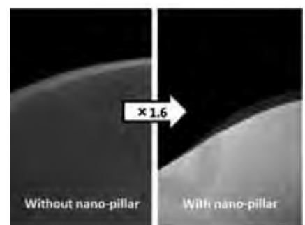
Fig.5 Comparison of antibody labeling intensity on health care chip
